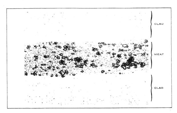
Fig. H-2 Photomicrograph of plate D-2321 away from ruptured edge (50x) (cross section).
