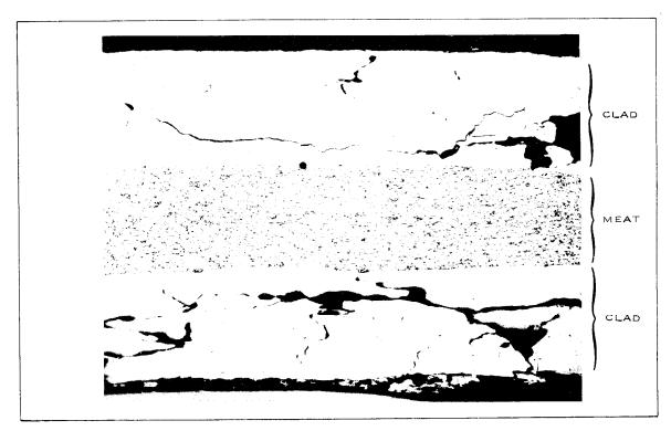
Fig. H-8 Photomicrograph of sample near the ruptured end of plate D-808 (50x).
