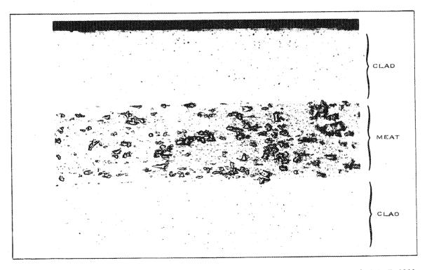
Fig. H-3 Photomicrograph of transverse-type specimen from the rupture area of plate D-2321 (50x).
