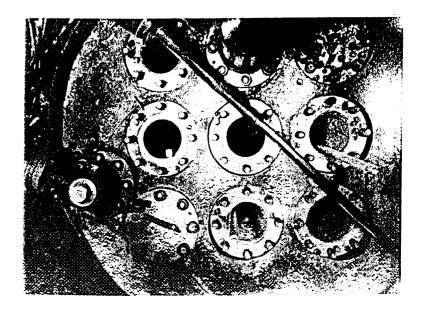
Fig. 27 View of SL-1 reactor vessel head after incident
