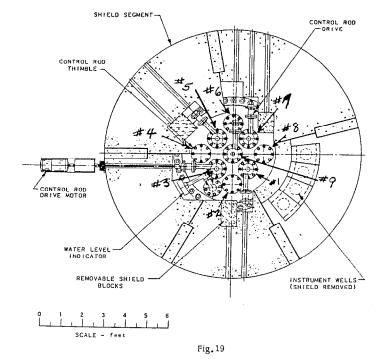
Control rod drives and top shielding
