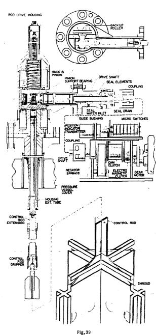
SL-1 control rod drive mechanism
