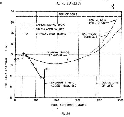
Critical rod bank position with equilibrium xenon concentration at 2,56 MW
