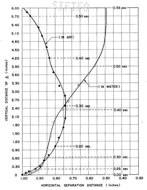
FIG. 7. Plot of the relative motion of <u>A</u> and <u>B</u> during scramming action, in air and in water, as read by comparator from Fastax camera traces.
