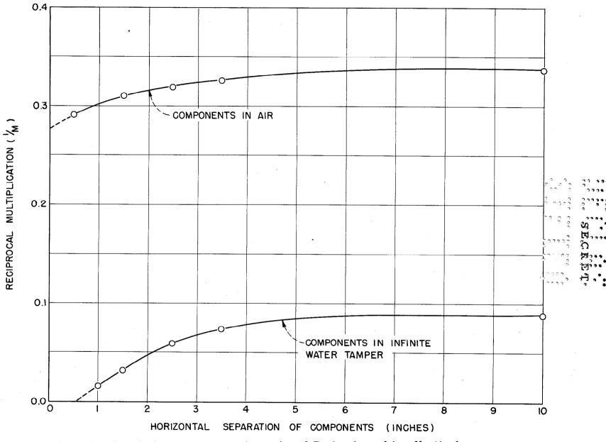
FIG. 3. Proximity measurements on <u>A</u> and <u>B</u>, in air and in effectively infinite water tamping.
