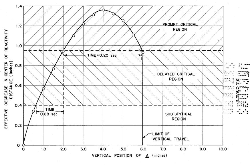
FIG. 8. Plot showing the combined effect of Causes (1), (2), and (3).
