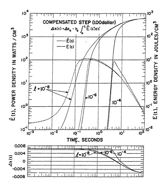
Fig. 8. Energy model computation of power versus time for an initial reactivity of 1.0 dollar above delayed critical for three different neutron lifetime values,  $\ell = 10^{-8}$ ,  $10^{-6}$ , and  $10^{-4}$  sec. Below are the corresponding curves of reactivity versus time.
