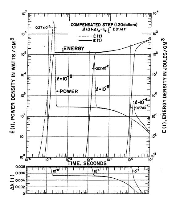
Fig. 7. Energy model computation of power versus time and energy release versus time, for an initial reactivity of 1.2 dollars above delayed critical for three different neutron lifetime values,  $\ell = 10^{-8}$ ,  $10^{-6}$ , and  $10^{-4}$  sec. Below are the corresponding curves of reactivity versus time.
