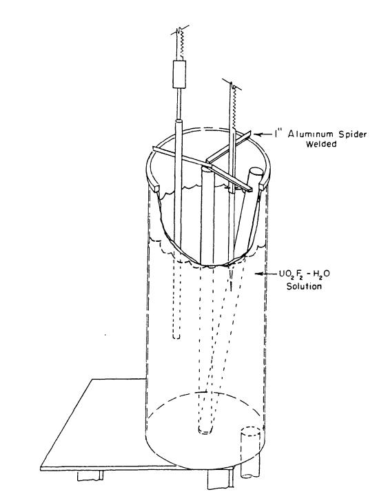
Fig. 1. The ORNL uranium solution assembly showing the normal and detached positions of the central poison rod.
