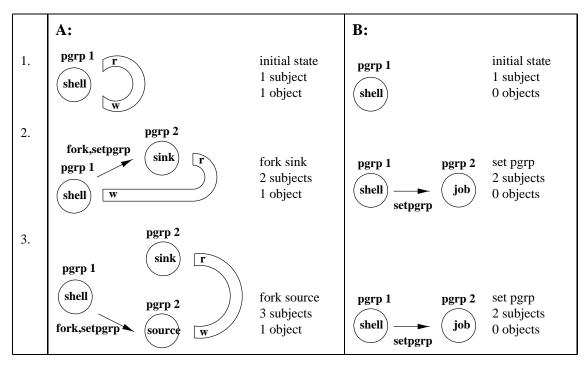
Figure 5. Simplified Representation of Shell Pipeline Behavior.
