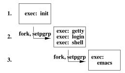
Figure 2. The UNIX login process tree
